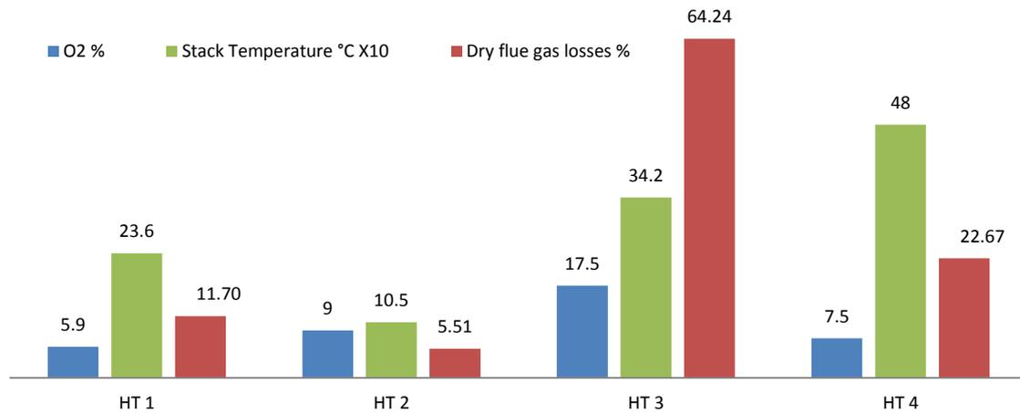
**Fig. 6.1 Relation Between Excess Oxygen, Stack Temperature and Dry Flue Gas Losses.**
