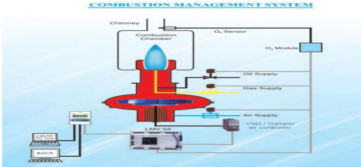
Fig. 8.1 Line Diagram of Combustion Management System
