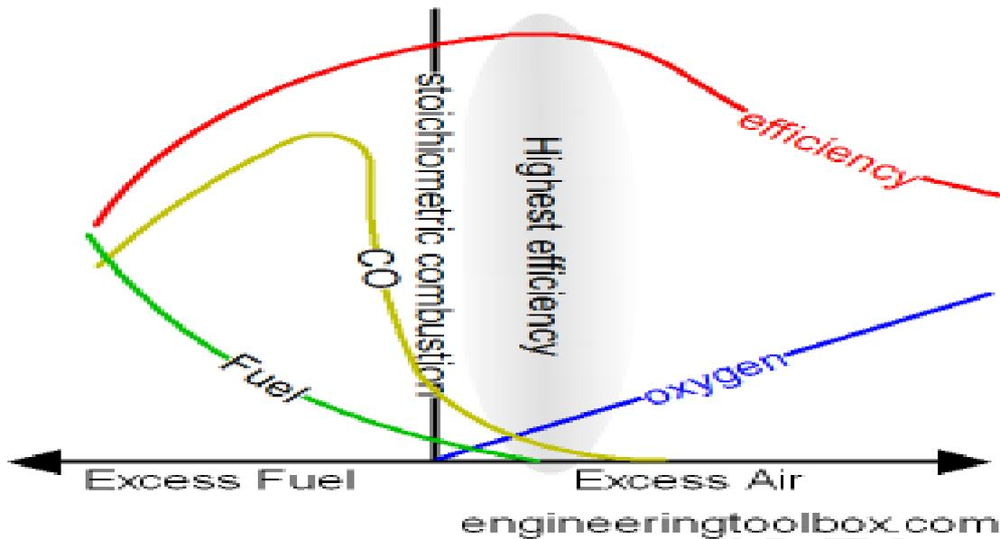
**Fig. 2.1 Efficiency vs Excess Air/Fuel Ratio**
